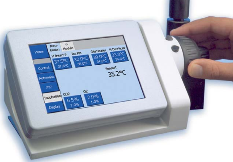
You can set all incubation parameters using the TFT touch screen display. The clear display showing setpoint and measured values allows perfect monitoring during the experiment
