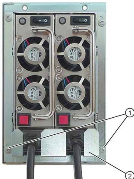
1. Remove the retaining screws ①.
