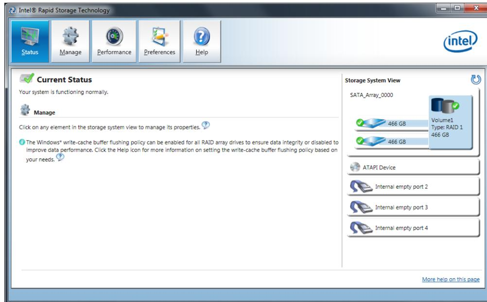
2. Select "Manage" > "Advanced" to display details of the RAID system.
