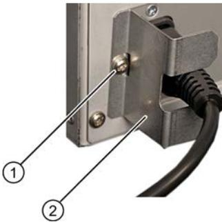
1. Remove the retaining screw ①.
