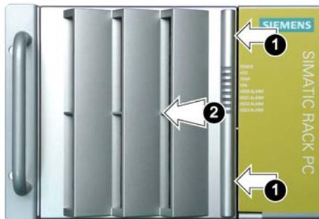
1. Press the marked at the same time to release the fan cover.
